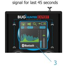
Displays the frequency of the signal or data transmission protocol identified
