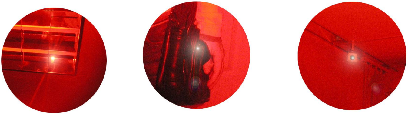
Figure 4 - view of camera flare in device's lens (a – camera hidden in a lamp; b – camera in a purse; c – CCTV camera in a store)
